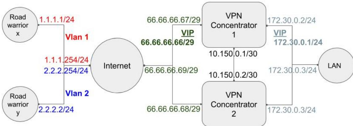
The key element in this use case is the VPN Concentrator. It should naturally have access to the resources located in the private network, on one hand; and access to the Internet, on the other hand.
